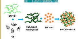
we developed a simple and effective strategy to fabricate carbon black(CB) based 3D hierarchical conductive structures in a natural rubber matrix using thiol-modified CNF(CNF-SH) as templates.
