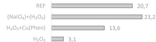
Figure 3. Energy consumption (MWh/t) for MFC production.
