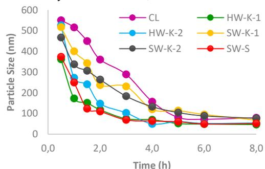
Figure 1. The average particle size observed during cellulose dissolution using DLS in the reference cellulosic substrates.
