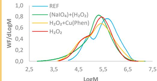
Figure 2. MWD after oxidation of HW-K-2
