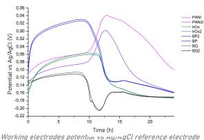
Norking electrodes potential vs Ay/AgCl reference electrode during bacteria growth in Bact/Alert culture medium
